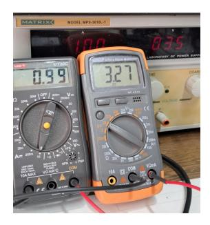
Testing MPPT algorithm, the power supply was set to 6V as per the MPPT value of the solar panel. The maximum current that was set to be available from the power source was set to 1A. After connecting the depleted battery pack the maximum transfer of power (W) was only 3.23W this is 50% lower than what the Solar Panel can provide.
