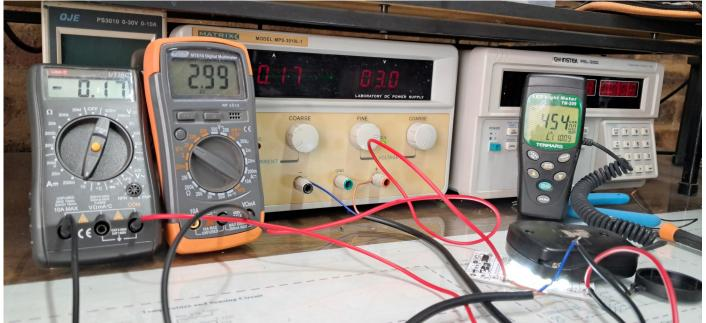
Run test 2.99V on battery Pack
